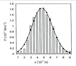
**Fig. 2.** Distribution of the surface power density of laser radiation fitted with a Gaussian function ( $\sigma = 1.56 \ 10^{-2} \text{ m}, x_{\text{mean}} = 4.77 \ 10^{-2} \text{ m}, P_{\text{max}} = 16.5 \ 10^{-2} \text{ W m}^{-2}$ ).
